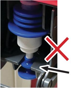
Incorrect. The Blue section is entirely beneath the Grey section.
