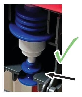
Correct. The Blue section is slotted between the Grey section.
