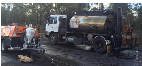
Bitumen tanker – Step One > clean down with BiCarb soda abrasive wet blast
