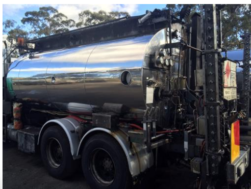
Bitumen Tanker – Step Two > after BITUSOL applied & washed down
